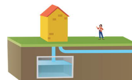
Booster Pumping Station & In-ground Storage Tank
