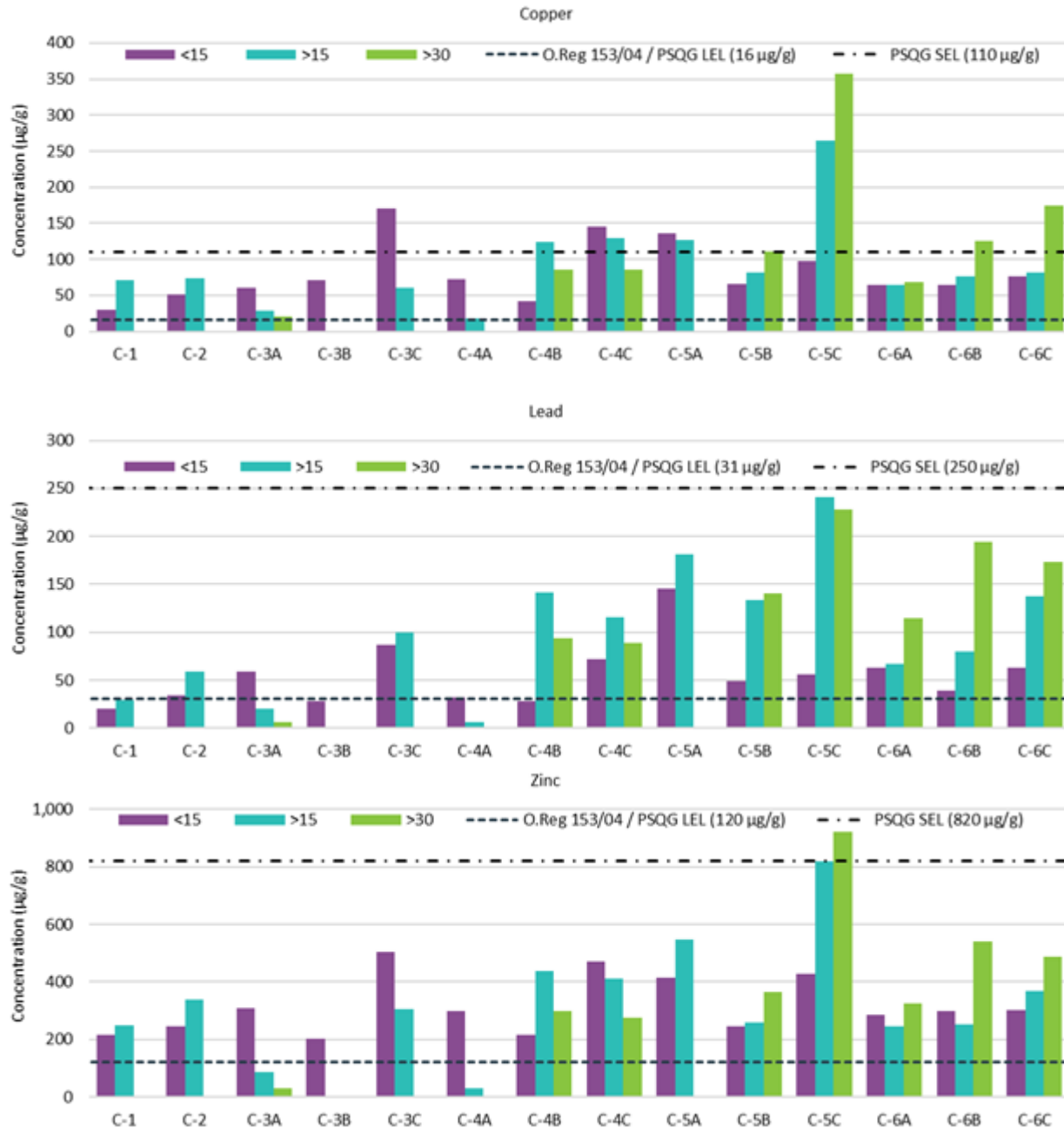
Figure 2.16. Copper, Lead and Zinc Concentrations in Chedoke Creek Sediments
